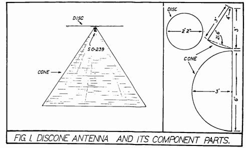
just a wee bit less than .5 inch. To get the proper spacing on mine, I had to mount the lid out on the end of the socket center-connector.
